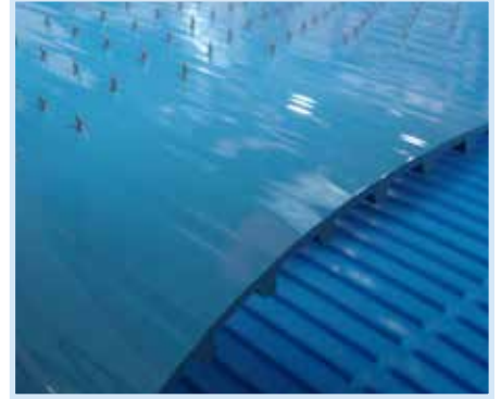
DualDrive™ Small Pulley with Metal Spikes
